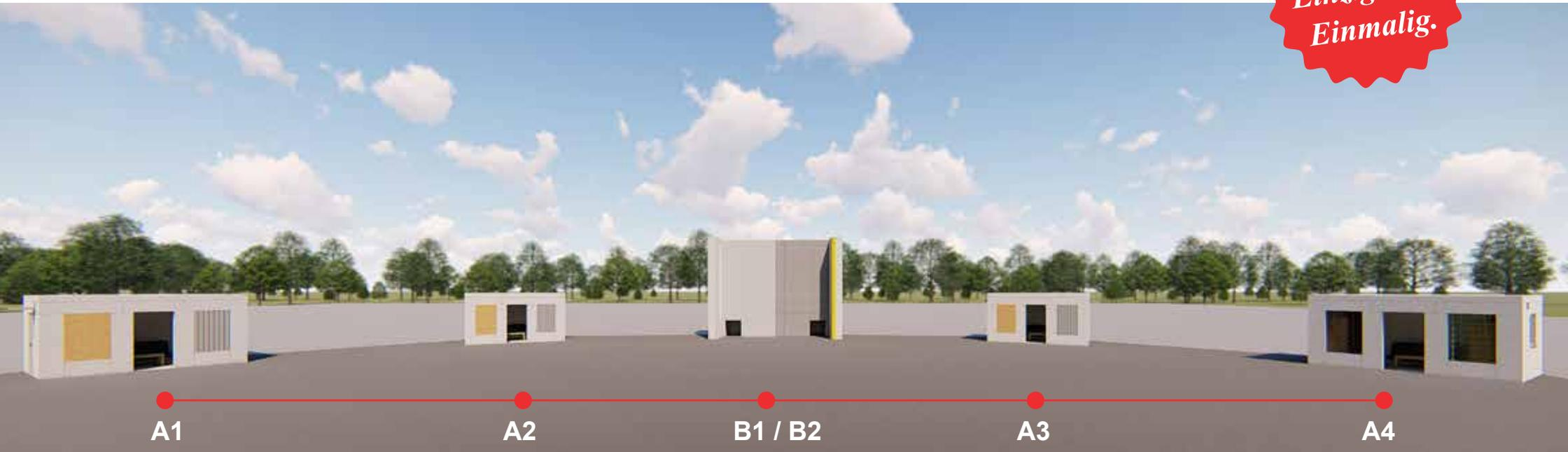
6 LIVE-BRANDVERSUCHE | BRANDRÄUME AUS PORENBETON 4MX5M | FASSADENNACHBAU MIT 6 METER HÖHE
