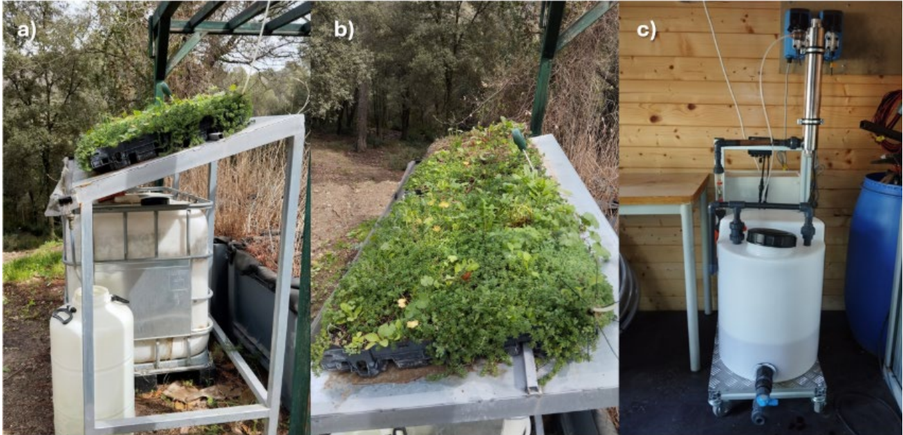
Figure 11: INFINITE Green roof set up. a) artificial roof with the modules above and the collection tank below. b) modules with sedum plants. c) disinfection UVC lamp and collection tank below. (© LEITAT)
